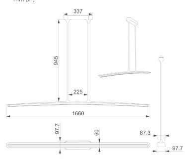
Reference SUYI1600LI Description Patinated bronze body - Alabaster diffuser - Protective varnish Reparability Driver and led are replaceable
