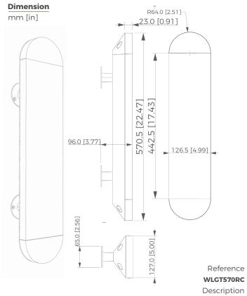
Patinated bronze body - Alabaster diffuser - Protective varnish Reparability Driver and led are replaceable
