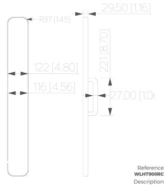
Patinated bronze body - Alabaster diffuser - Protective varnish Reparability Driver and led are replaceable
