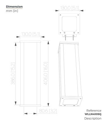
Patinated bronze body - Alabaster diffuser - Protective varnish Reparability Driver and led are replaceable
